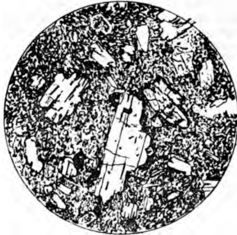
FIG. 19.—ANDESITE WITH PORPHYRITIC HYPERSTHENE AND FELSPAR ; Moel-y-Golfa, Breiddens, x. 25.
